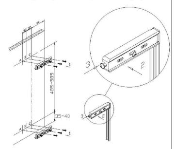
Adjusting closure pitch of cabinet door by the door mounting bracket, then fixup all screws. (Pay attention to assembly swivel arm, for left and right mounted door mirror image)
