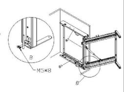
Step 4:Connect side frame and rear slide frame by swivel arm, and firm door mount bracket on pull-out side frame.
